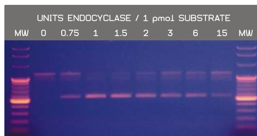
Fig.3: Processing of a 1 kb PCR product with a central recognition site into two 500 bp DNA fragments, which are covalently linked at one side. Endocyclase N15 processing efficiency is highly dependent on the amount of enzyme. Best results are obtained, when exactly 1 U of enzyme is used per pmol of DNA.
